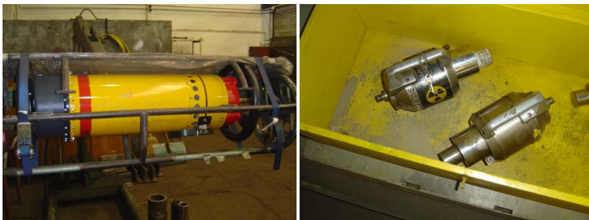
Figure 18: An X-ray machine and defectoscopes used in industrial radiography. (Photo: SNSA inspectorate)
