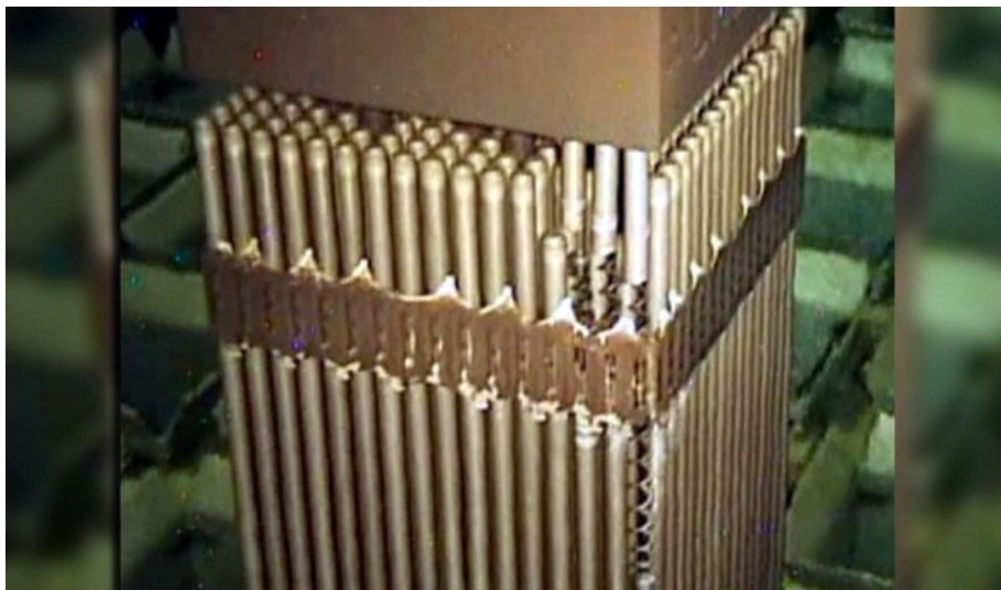
Figure 13: Damaged fuel assembly AD11 (Source: Kanal A)
